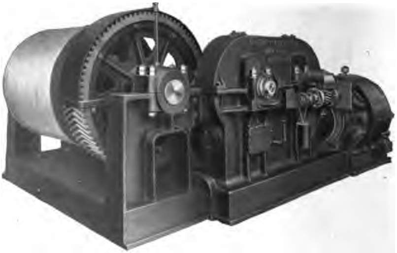
Fig. 169. Tandem-Gear Elevator with Herringbone Reduction Gearing Courtesy of Gurney Elevator Company
